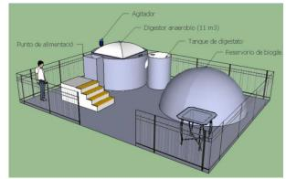
Once location is selected, engineers from the Company VIOGAZ, which will be subcontracted to design and build the biodigestor, will proceed with the design's math regarding grease production projections coming from the grease traps of the involved food sector businesses. They will then list the necessary materials and equipment according to the design. Preliminary estimations indicate a capacity of 3.1 m<sup>3</sup> with a 75 day hydraulic retention time.
