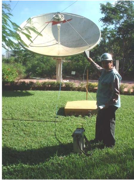
This method uses a spectrum analyzer and a horn antenna operating in the frequency range of interest, which for this type of verification would be the transmission frequency to the satellite in the corresponding operation band.
