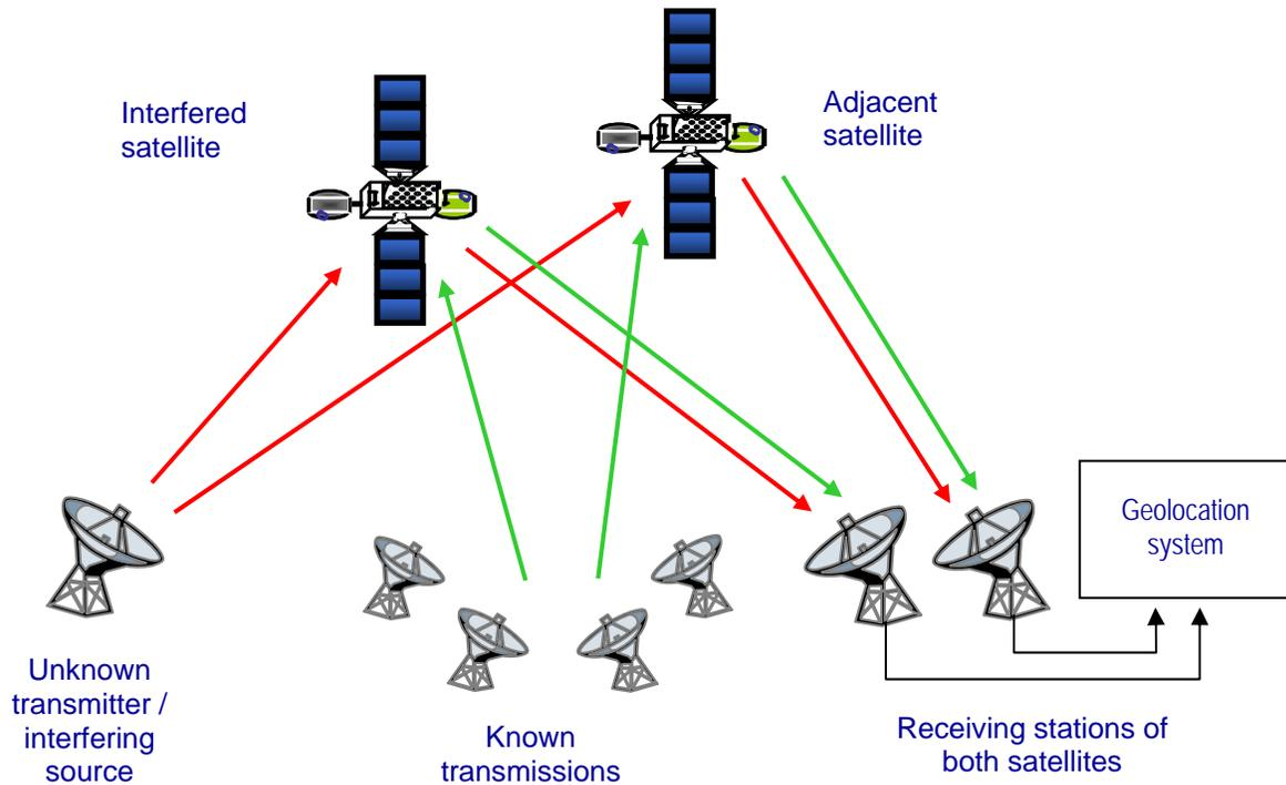
The unknown transmitter antenna is aimed at the interfered satellite, transmitting most of its energy through the main lobe and a smaller part of its energy through the side lobes, which reaches adjacent satellites at a very low level.
